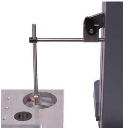
Internal groove measurements with accessories 54-199-508, 54-199-506 and 54-199-501
