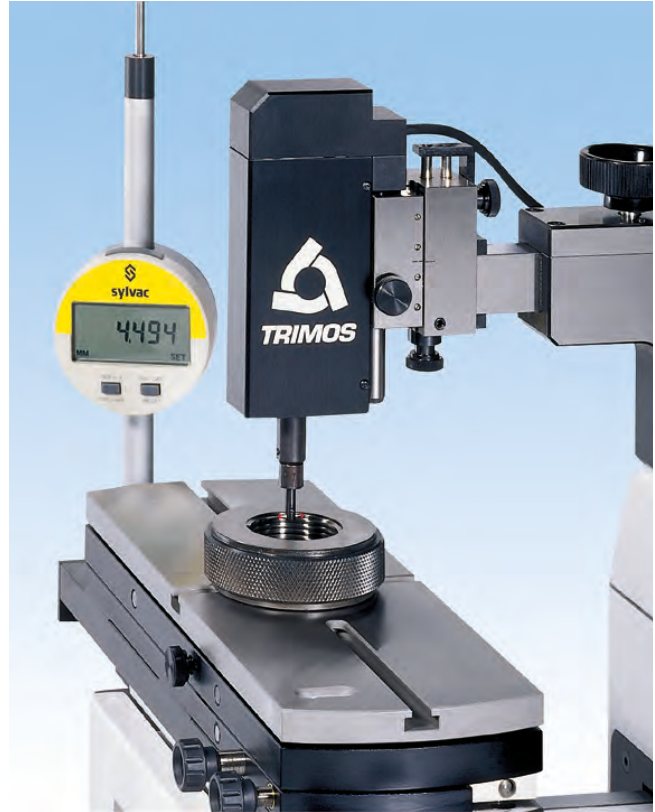
▲ Checking of threaded ring gages from pitch 0.7 to 6mm/48 to 4 threads per inch (max. internal dia. 7.08"/180mm) using table (54-197-011), clamps (54-197-142), Internal measuring device (54-197-074) & T-Ball probes (54-197-075)
