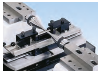
Checking of plug gages and threaded plug gages between centers up to max. dia. 1.18"/30mm, max. length 6"/150mm using table (54-197-011), small Ø anvils (54-197-806) & thread wires (54-197-007)
