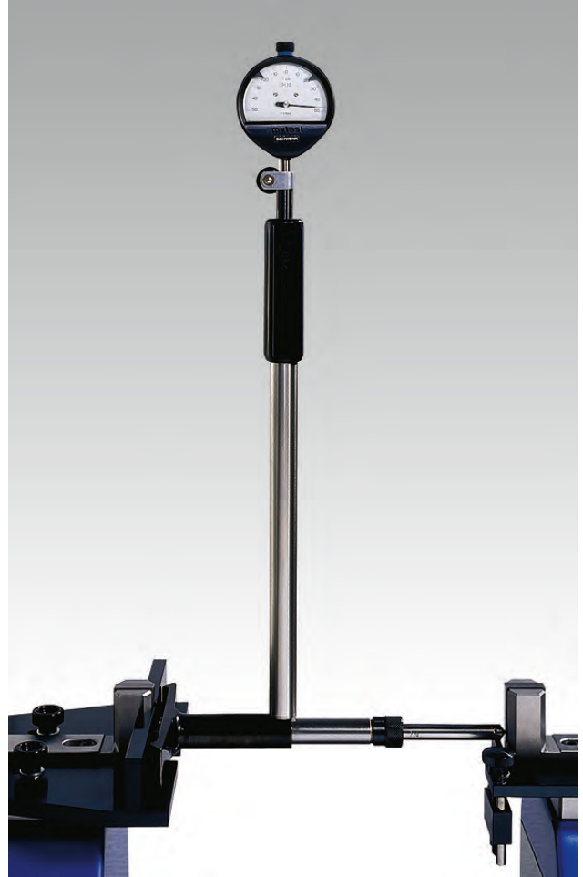
▲ Setting of 2-point bore gages using gage block anvils (54-190-805), bore gage centering supports (54-190-829) and secondary contact support (54-196-040)
