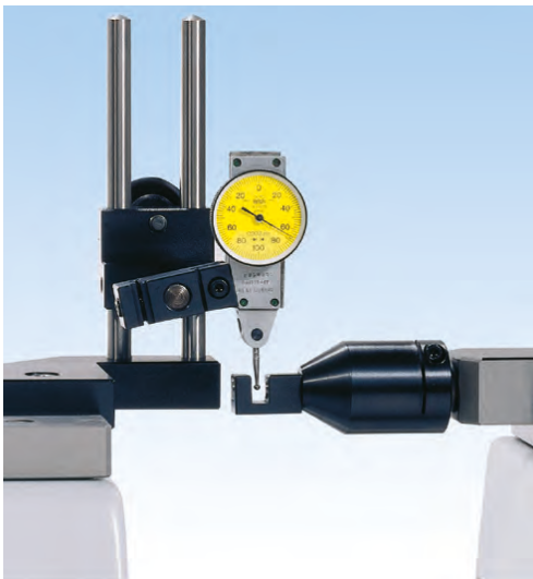
▲ Checking of lever (test) dial indicators using 54-197-115
