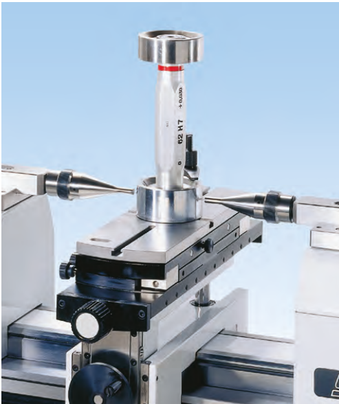
▲ Checking of plug gages and threaded plug gages from dia. 1.18" to 10"/30 to 250mm using table (54-197-011), clamps (54-197-142), small Ø anvils (54-190-806) & thread wires (54-197-007)
